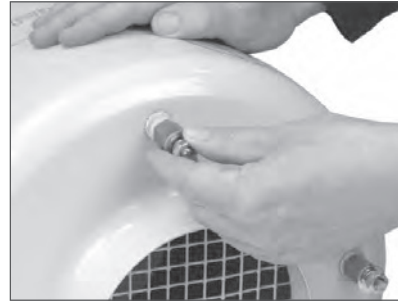
(2) Fit 4 x case studs (supplied with unit).
