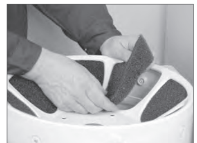
(12) Remove old silencer & fit new silencer.
