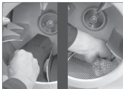
(5) Remove old drum pads, clean inside of drum and inspect drum for signs of damage.
