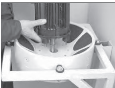
(10) Withdraw motor from housing.
