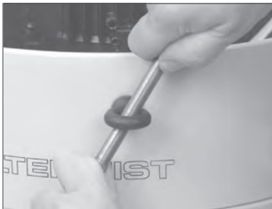
(3) Tighten eyebolts until horizontal.
