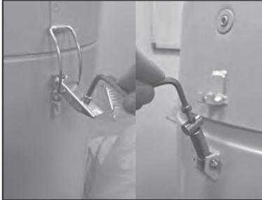
(1) Undo safety latch and clips.
