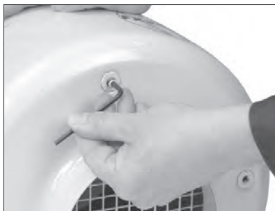
(1) Fit case studs as for Direct Mount.
