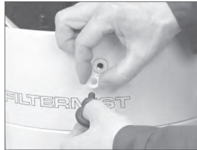
(2) Screw in 4 x eyebolts with nylon washers.
