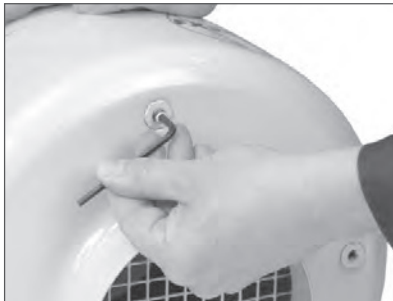
(1) Remove 4 x insert screws in base of unit.
