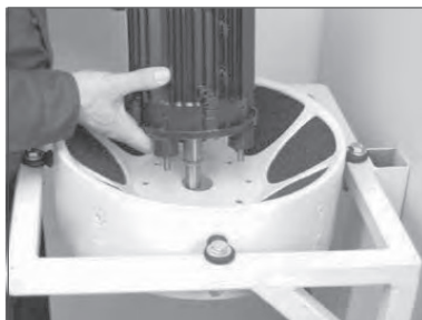
(13) Re-fit motor to top of case.
