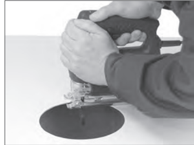
(4) Cut extraction hole in machine enclosure.
