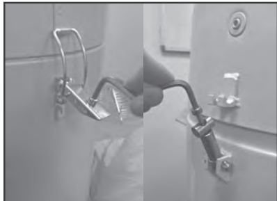
(1) Undo safety latch and clips.
